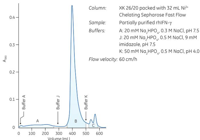
**Fig 3.** Partial purification of rhIFN-γ on Chelating Sepharose Fast Flow. Activity of rhIFN-γ was localized to peak B, which was pooled for final purification on Superdex 75 prep grade. Reprinted from Zhang, Z. *et al.* (3).
